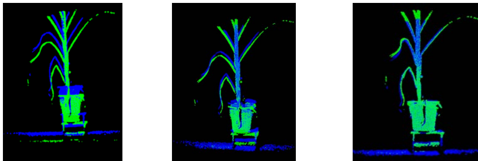
(a)Original point cloud (b) ICP Registration algorithm (C) Registration algorithm in this paper
